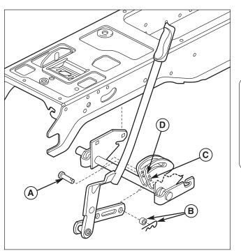
Figure 20. Lift Link Positions-Normal
